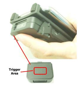
The touch trigger is in the central area of mini scanner. (for both side). Please check the above drawing for your reference.
