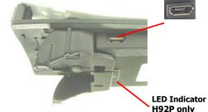
H92P Scan Holder is with Li-Ion battery inside. When in charging, please use the original power adaptor of smartphone (recommend). Through it, it charges both OTG device and H92P internal battery at the same time. When in low battery (Red LED flashing), please charge it immediately.
