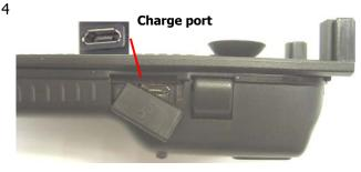
DC9270 is with Li-Ion battery inside. When in charging, please use the original power adaptor of OTG device (recommend). Through it, it charges both OTG device and DC9270 internal battery at the same time. When in low battery (Red LED flashing), please charge it immediately.
