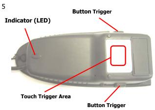
The touch sensor area is around the central area. There are 2 button triggers on the right and left side.
